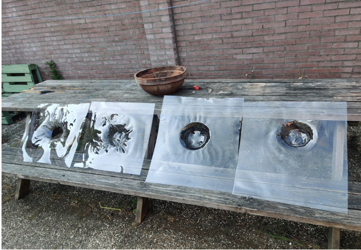
Figure 19, To create the shape of the dashboard I needed to hand form polyester sheets as a vacuum former was too small. This cost 4 iterations.
